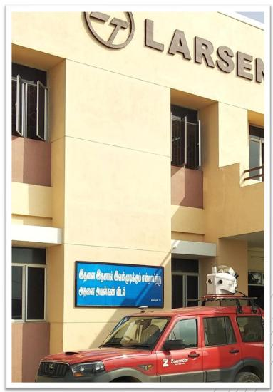
Mobile LiDAR Uses Laser Scanners In Combination With GNSS Receivers, IMU And a DMI. It Acquires Accurate And Precise Spatial Data With Six To Eight Cameras On Any Vehicle.
