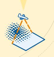
LiDAR that stands for Light Detection and Ranging is a technology that is based on laser beams. It shoots outs laser and measures the time it takes for the light to return. It is so-called active sensor as it emits its energy source rather than detects energy emitted from objects on the ground.
